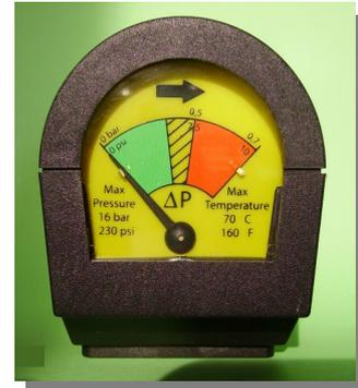
The measure of differential pressure allows to identify when the change out of the filter element is **suitable and convenient**. The pressure gauge has on both side a scale in two colors in the range from 0 to 0,7 bar.
