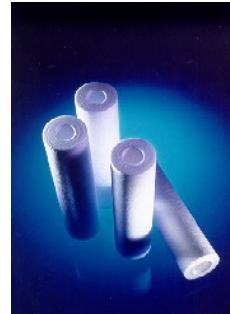
STARLIFE is a depth filter integrally manufactured with polypropylene. The filter media is obtained by Melt-Blown process technology; the microfibers with a precise and controlled diameter are thermally bounded in order to obtain a porosity decreasing from external, to obtain high dirt holding capacity with low filtration cost. The strongly bounded microfibers provide high resistance to pressure drop increase and preserve constant flow rate.
