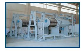
Photo shows an horizontal leaf filter; the extraction of leaves package as well as the opening of bayonet quick closure is hydraulically done.
