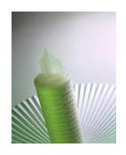
POLYSAN-PKP is obtained by pleating up to 5 polypropylene layers of decreasing porosity to achieve high effective filtration area, high dirt holding capacity and precise and controlled filter ratings.
