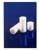
POLYSAN MINI-CARTRIDGE is obtained by pleating up to 5 polypropylene layers of decreasing porosity to achieve high effective filtration area, high dirt holding capacity with efficiency higher than 99.98%.
