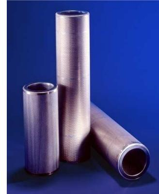
The DUALSEP filter elements are manufactured using a pleated structure made with two different layers: the external layer provides high dirt holding capacity; the internal one agglomerate the mist in larger drops.
