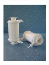
QUALIKAP QKP-C capsules are specifically designed to use the positive charged nylon 6,6 membrane . QUALIKAP QKP-C greatly interacts with the negative particles contained in the liquid in order to withholds particles smaller than the pore size. QUALIKAP QKP-C have proven to hold a great quantity of submicron particles and endotoxins.
