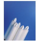
POLYSAN-PKN is obtained by pleating several polypropylene layers of decreasing porosity to achieve high effective filtration area, high dirt holding capacity and controlled filter ratings.
