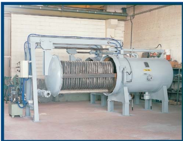
Photo at the left shows an horizontal leaf filter; the extraction of leaves package as well as the opening of bayonet quick closure is hydraulically done.
